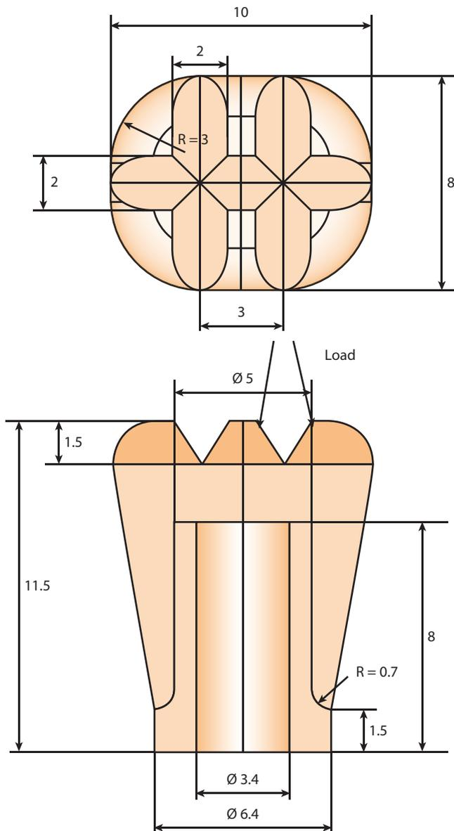
**Figure 2.** Digital design of crown on abutment as used in static loading test for FEA (dimensions in mm).
