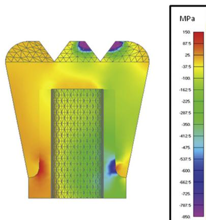
**Figure 5.** Solid Y normal (vertical) stress on lithium disilicate crown fixed to titanium abutment with peak in cervical area (model 1).
