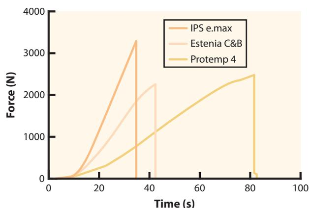
**Figure 4.** Stress-time curve of ILF experiment.
