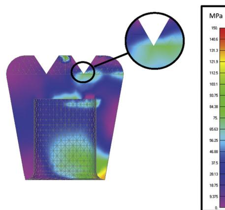
**Figure 7.** Solid maximum principal stress (tensile stress) on lithium disilicate crown with contact surfaces in interface crown/abutment (model 2). Highest stresses were found in fissure and beside top of abutment.
