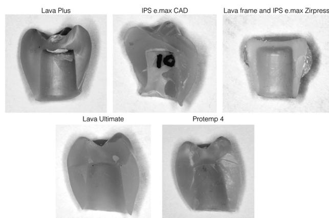
**Figure 3.** Remnants of fractured specimens after ILF test. Mist and hackle area in occlusal part of fractured LP and PT crowns demonstrate that fracture originated from fissure.
