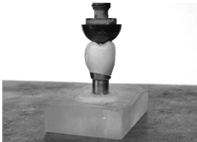
**Figure 1.** Arrangement used for ILF test.
